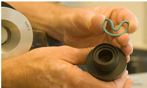
Figure 3.3 Split Groove Piston Seal Installation
