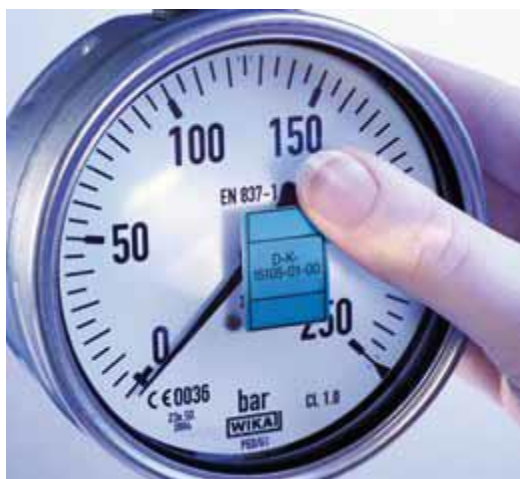
Fig. 5.4: Calibration sticker on a mechanical pressure gauge
