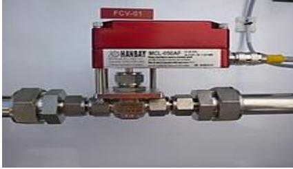
Figure 4.8 Electric valve actuator controlling ½ needle valves
